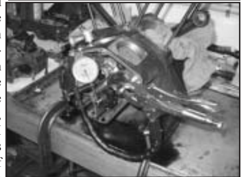
Checking Pinion Shaft Run-out
