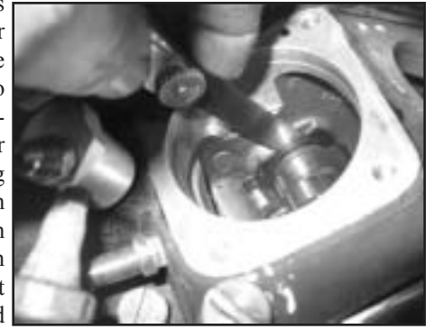
Check the camshaft end play prior to removing the cam cover.
